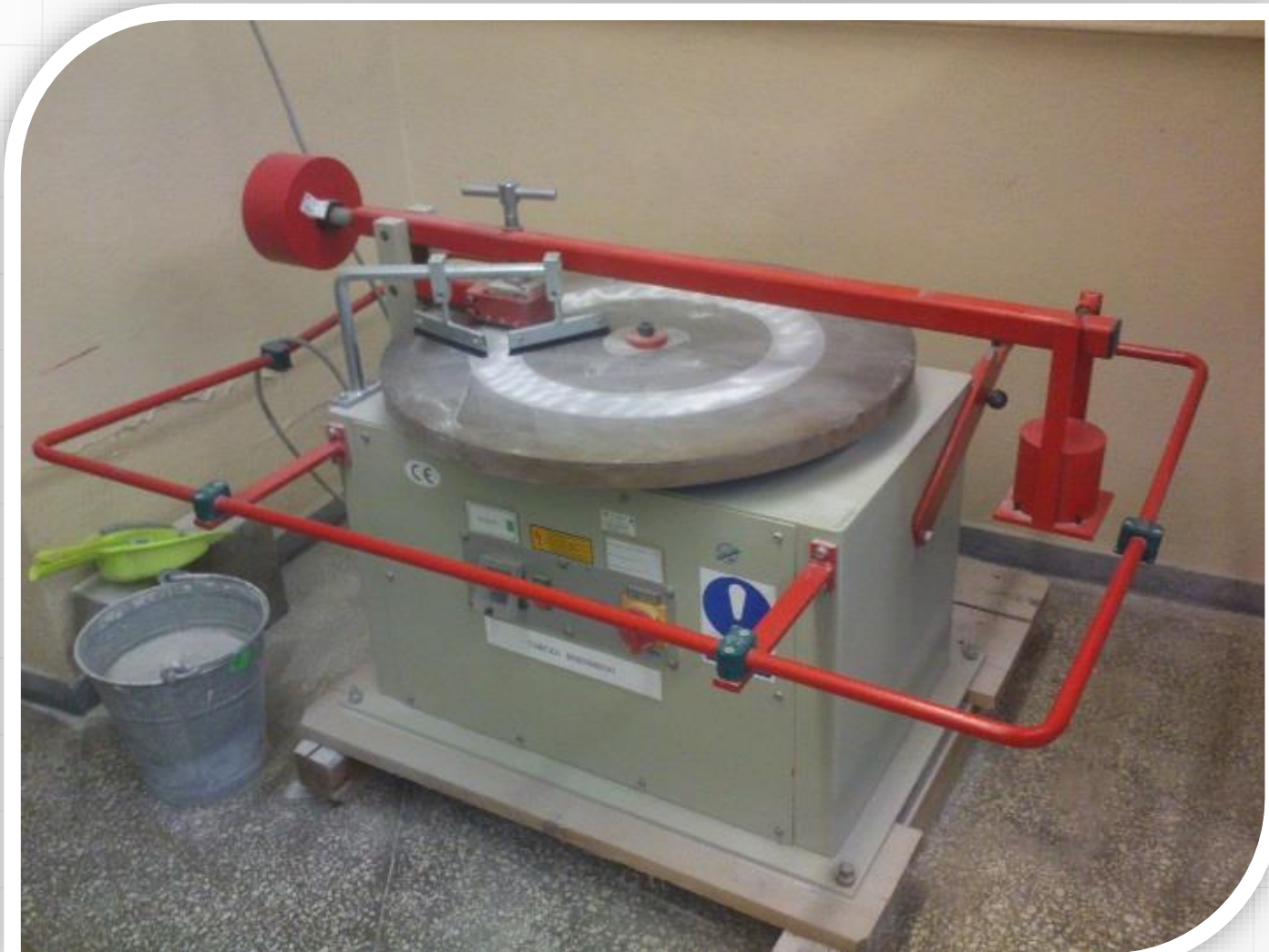
View of the test bench for testing abrasiveness on the Boehme disc
