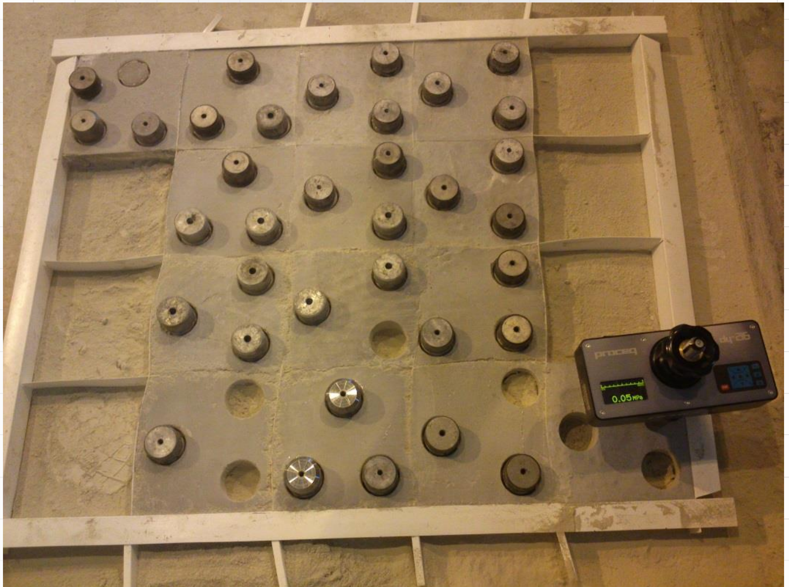
View of the surface of the overlay after the pull-off tests
