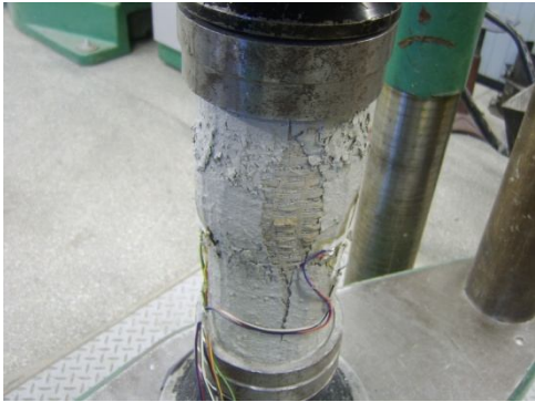
Fig. 6. Image of destruction of the element reinforced with two layers of PBO mesh [32 in Z6]
