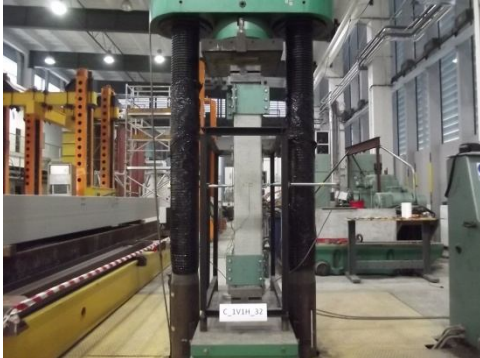
Fig. 29. Element on the 32 mm eccentricity ( h/6 ) at the test bench [36 in Z6]
