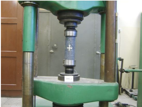
Fig. 1. Element reinforced with one layer of CFRP sheets on the test bench [32 in Z6]
