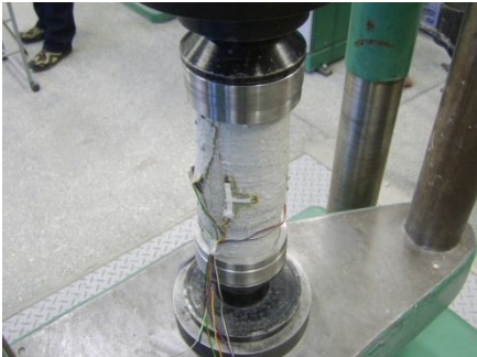
Fig. 25. Paths of transverse strains as a function of the load and the image destruction of the 20M2_1 element [35 in Z6]
