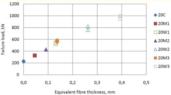
Fig. 3. Limit load-bearing capacity (failure load) elements without prior exposure to temperature [32 in Z6]
