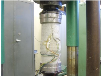
Fig. 26. Paths of transverse strains as a function of the load and the image destruction of the 20M3_2 element [35 in Z6]
