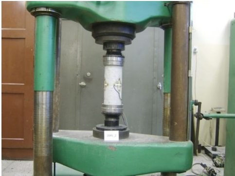
Fig. 2. Element reinforced with one layer of PBO mesh on the test bench [32 in Z6]
