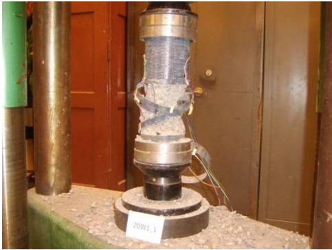
Fig. 5. Image of destruction of the element reinforced with one layer of CFRP sheet [32 in Z6]
