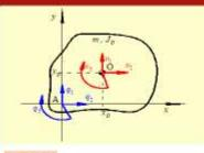
This is the plane rigid body, which mass is m and polar mass moment of inertia about the axe through the mass center point  $J_{\sigma}$  is given. The example shows haw to determine a mass matrix in the generalized coordinate base.
