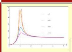
The transmissibility  $\nu_T'$  as a function of frequency ratio for various amounts of damping
